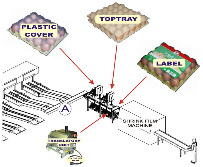
The DISPENSERS GROUP is linked to 4 takeaway lanes and is able to feed a SHRINK FL M machine at the rate of 40 trays / mn
